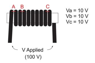
Higher inductance parts have higher number of turns. Voltage capacity of the inductor to resist breakdown depends on the wire insulation to withstand turn-to-turn voltage stress.
